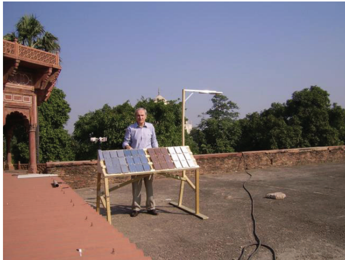
The Malé Declaration has produced new dose-response functions for carbon steel, zinc, copper and limestone for South Asian conditions
