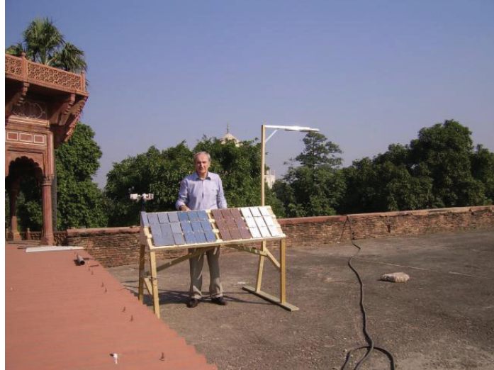
Figure 2.3.2. The corrosion rack and the covered passive sampler exposure mount at the Agra site in India (Taj Mahal is behind the trees).
