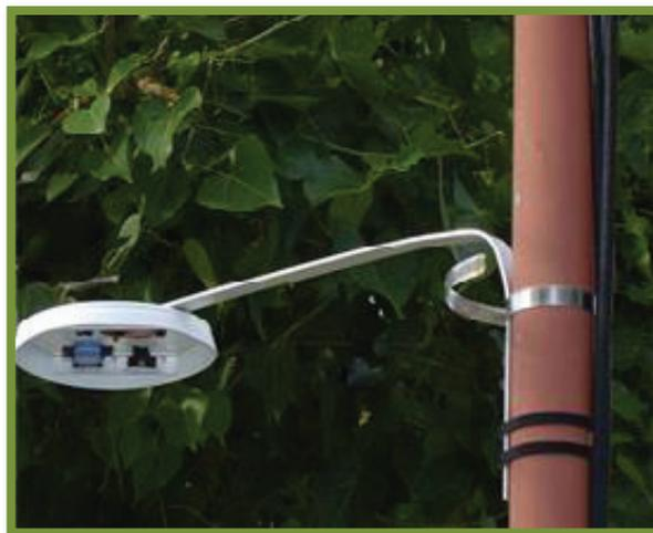
**Figure 2. Samplers mounted under rain shield**
