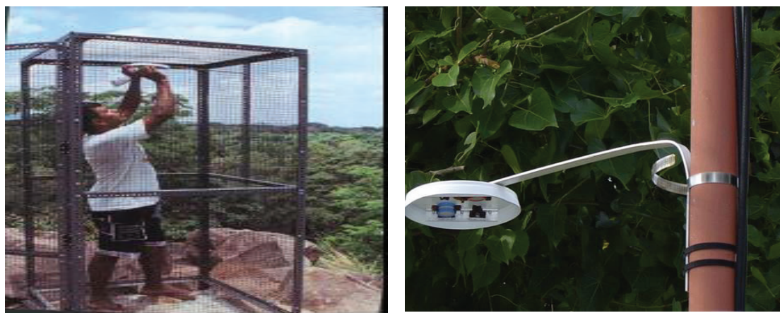
Figure 2-22 Diffusive samplers at a Malé station
