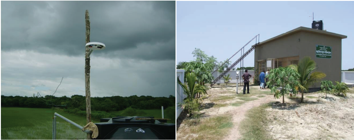
Figure 2-2 Passive Sampler; Station with bulk sampler
